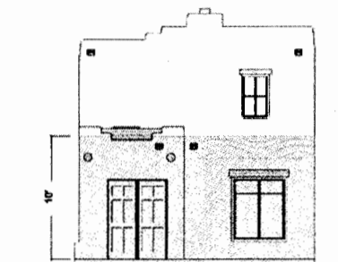
Surface Area of Doors and Windows must be at least 25% of total hatched area
