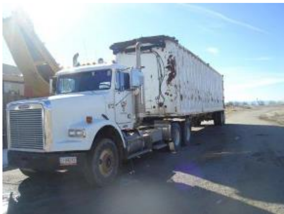
Figure 2-13. Transfer Trailer and Roll-off Truck
