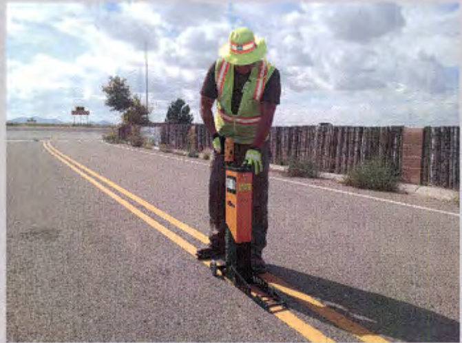
Picture - ( R ) Carlos Casisas, Santa Fe County Traffic Mobility Technician using the Retro reflectometer on County Road 62 and County Road 68A.
