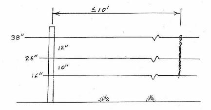
Figure 2. Recommended 4-strand fence with nearly-equal wire spacings. Top and bottom wires are best if smooth, rather that barbed. This is more critical for the top wire. Fence posts and stays should be no more than 10 feet apart, to keep a taut fence. Wires should be at 16, 22, 28 and 38 inches above ground to accommodate crawling and jumping animals.
