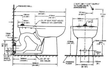
**DIMENSIONS (Nominal)** NOTE: Distance from floor to closet flange centerline (rough-in) must be 4\* (102 mm) with flange surface flush to 1/16\* (1.6mm) max. beyond finished wall.
