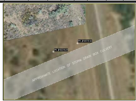
Remarks: Pothole on Storm Drain Box Culvert as directed. Second attempt at relocated location north of the original location (PH 102319.01). Cleared pothole to 36".
