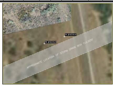
Remarks: Pothole on Storm Drain Box Culvert as directed. Cleared pothole to 84".
