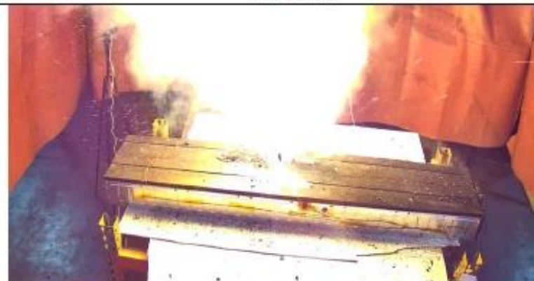
(h) Second propagation After Initiating Cell (Cell 31) 1:13:49
