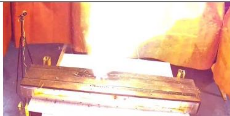
(g) First propagation after Initiating Cell (Cell 35) 00:58:04
