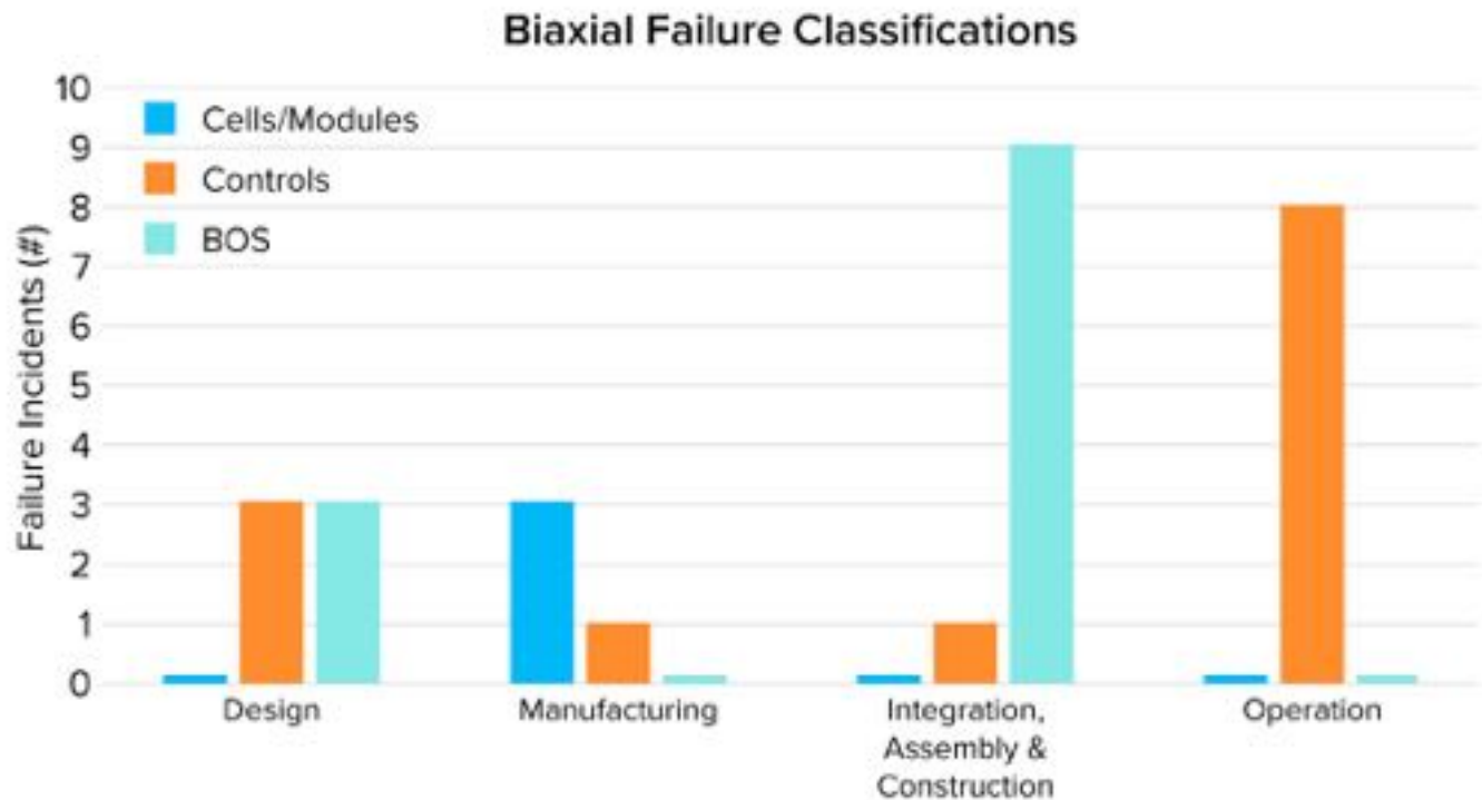
Figure 7. Relationship between Root Cause and Failed Element
