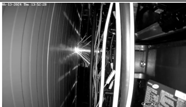
Figure 2.9: During cell venting (Time in 13:52)
