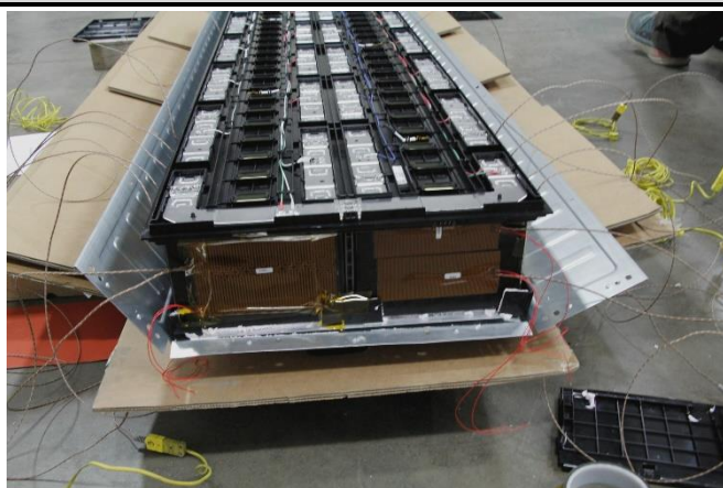
Figure 2.6: Location of primary (left) and secondary (right) film heaters on Cells 1 and 2, respectively
