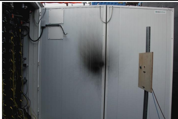
Figure 2.15: After test initiating module soot
