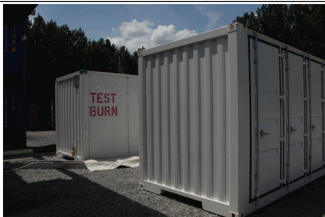
Figure 2.3: Initiating and target containers sealed and in the test area
