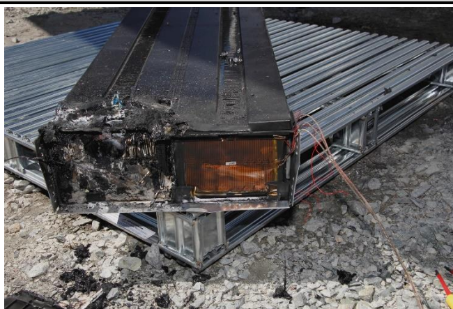
Figure 2.7: Pre-Test conducted on single module to confirm propagation from Cell 1 to Cell 3, post test damage
