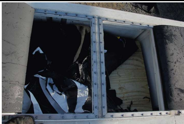
Figure 127: Inside of deflagration panel through roof after test 2 showing remains of gas containment vessel inside of DUT
