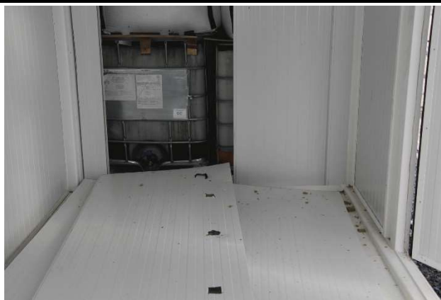
Figure 1.28: Inside of DUT after test 2 showing collapsed divider wall
