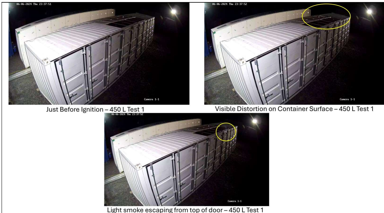
Figure 8: Container stress distortion and light smoke escaping from the door – Test 1
