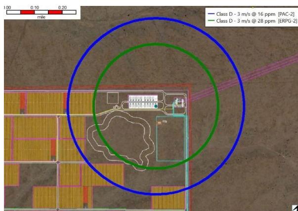
Figure 19 – Scenario #3 Toxicity Gas Cloud (Class D at 3 m/s Atmospheric Conditions) Top View at 135'-0" Height
