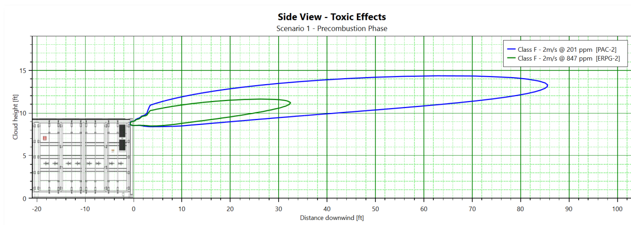
Figure 6 – Scenario #1 Toxic Gas Cloud (Class F at 2 m/s Atmospheric Conditions) Side View
