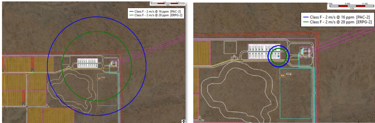
Figure 16 – Scenario #2 Toxicity Gas Cloud (Class F at 2 m/s Atmospheric Conditions) Left Image: Top View at 80'-0" Height, Right Image: Top View at 6'-0" Height
