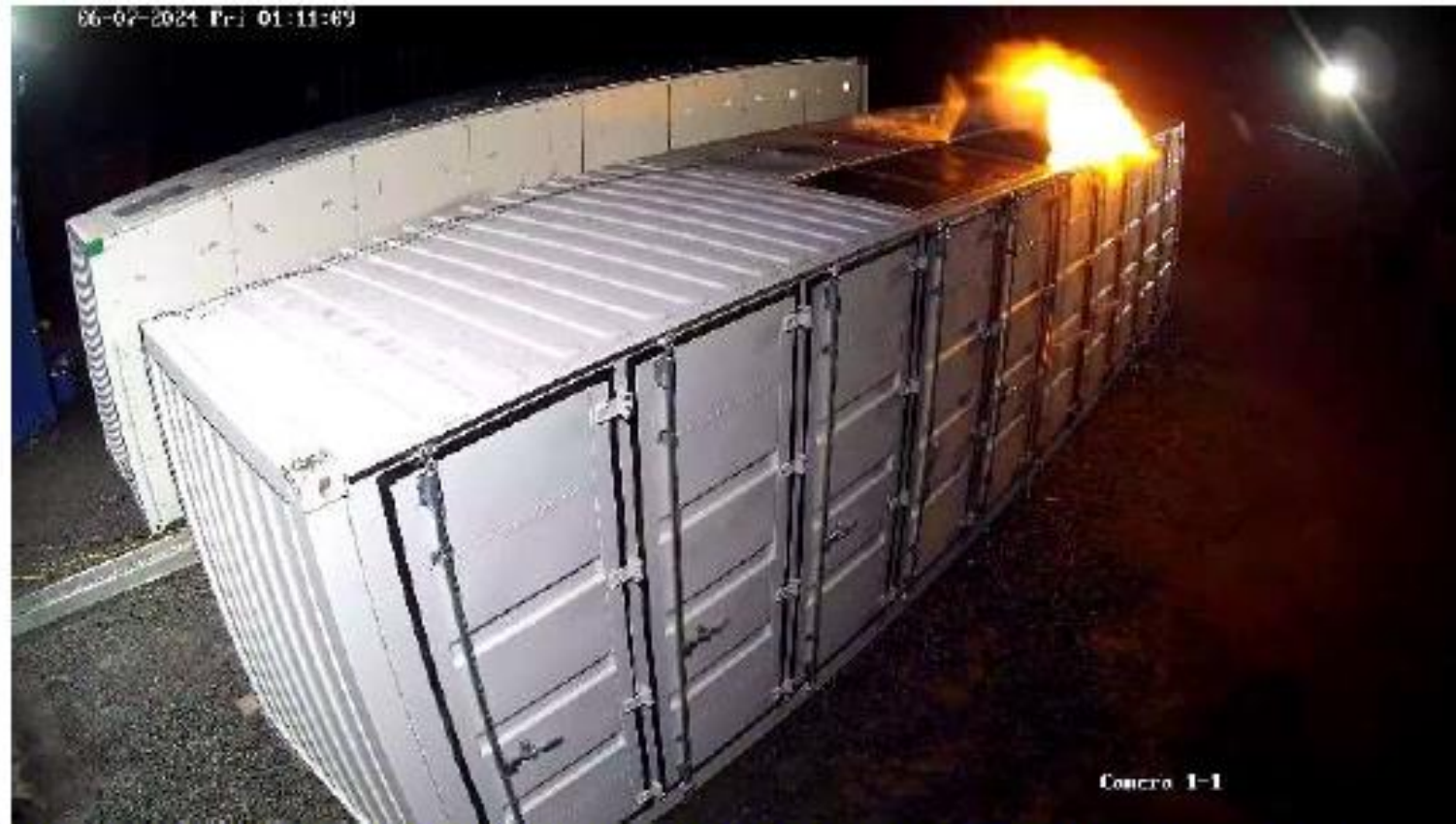
Figure 9: Flames ejected from deflagration panels as viewed from the rear of the container – Test 2
