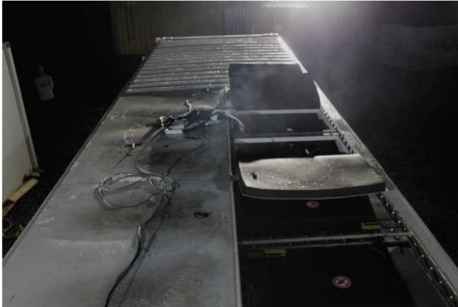
Figure 10: Deflagration panels post-test 2
