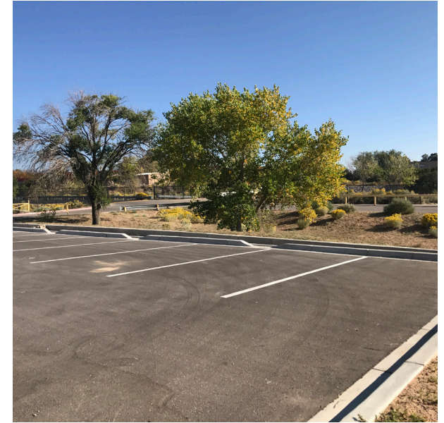
Figure 13. Numerous curb inlets along a median edge might promote better stormwater catchment than a singular opening. Extra curb cut openings are good where maximizing inflow is desired, where unevenness of gutter or adjacent impervious areas might require multiple inlets, or to prevent pooling water on parking areas if the curb is on contour (i.e. minimal slope).captured.
