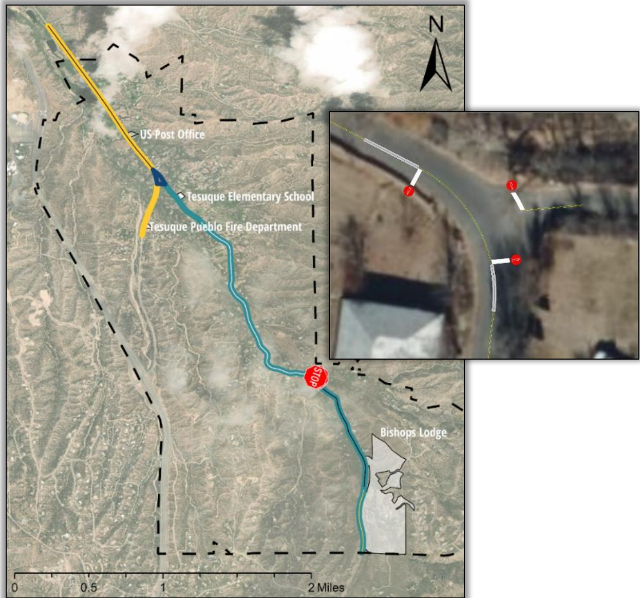
Figure 49: Conceptual drawing of All-Way Stop Control at Bishops Lodge Road and Big Tesuque Canyon
