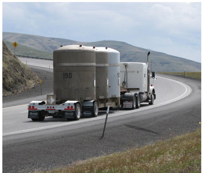
Each TRUPACT-II holds up to fourteen 55-gallon drums.
